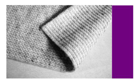
Characteristic: Nonwoven textile mechanically bonded by stitchingMaterial content: PP staple fibers FIBROSAN for sorption of oil products
