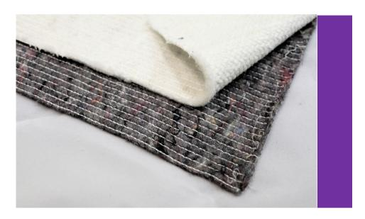
Characteristic: Nonwoven textile reinforced mechanically by needle punching
